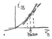
This represents a <u>linear time-variable</u> conductance  $\hat{g}$  in  $\hat{N}$ . (Time-variable, since  $\partial i_B/\partial V_B$  varies in N in time, even if the  $i_B$ - $V_B$  characteristic is time-invariant, except of course for DC circuits.) Or for small signals!
