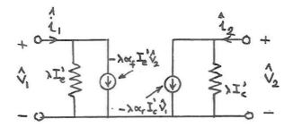
Since  $I'_e = f_1(v_e)$  &  $I'_c = f_2(v_c)$ , the elements in this linear twoport vary with the voltages in N. Hence, N must be analyzed before  $\widehat{N}$ ; then  $\widehat{N}$  is easy to analyze, since it is linear.
